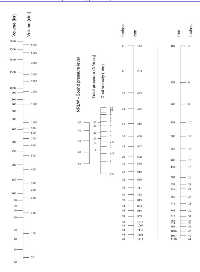
When using an SD grille for supply, refer to DD nomogram for figures. Sound power & pressure levels are based upon exhaust air with dampers fully open. Without dampers subtract 2dB and multiply total pressure by 0.9.
