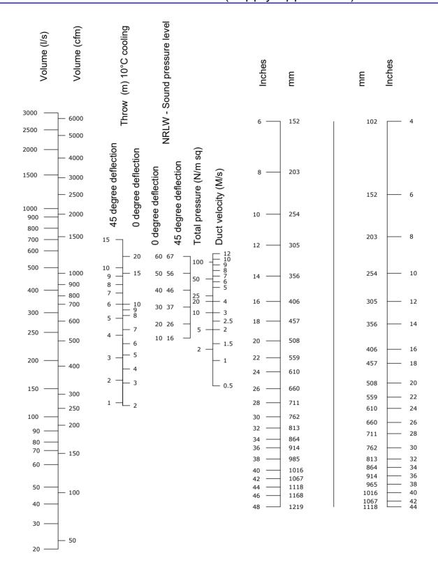
Throw values based on grilles mounted in sidewall not more than 1m below an unrestricted ceiling. For grilles positioned more than 1m below an unrestricted ceiling, reduce throw values by 25%. Sound power & pressure levels are based upon supply air with dampers fully open. Without dampers subtract 2dB and multiply total pressure by 0.9. Throw values based on a 10°C cooling application. For isothermal applications, increase throw values by 25%.
