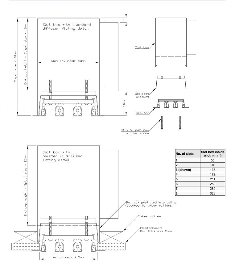
Slot boxes are supplied with brush seal strips fitted to end caps to reduce leakage from between the diffuser and the box.
