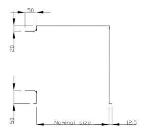
12.5mm flanges shown are used on boxes to suit all terminal series' except CD and PPD.
