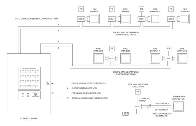
VFC = Volt free contact FS = Fused spur
