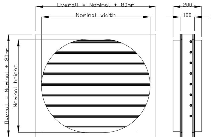
**Spigots:** Model B spigots supplied 6mm under nominal size.
